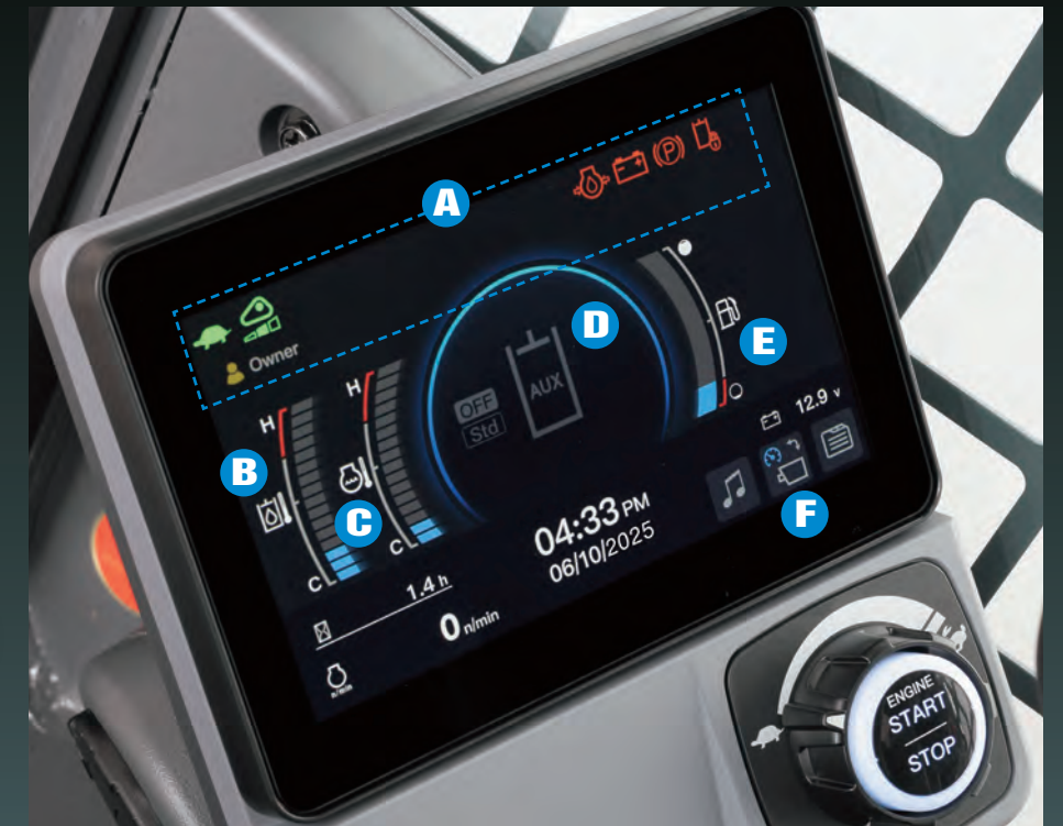
A. Situation Indicator (such as working function, battery charge indicator etc..) B. Hydraulic Oil Temperature C. Coolant Temperature D. AUX Mode E. Fuel Level F. Menu Icons
